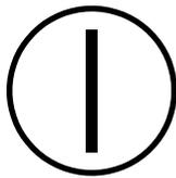
**ON** - Pressing this button will start up the UPS in order to provide conditioned and protected power.
